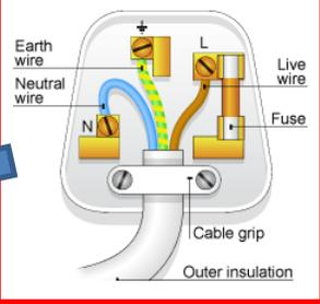
The circuits in your house are earthed outside. Appliances with metal cases need to be earthed inside the case. This is just in case a live wire comes loose- the current will then pass through the earth wire and not you when you touch it.
