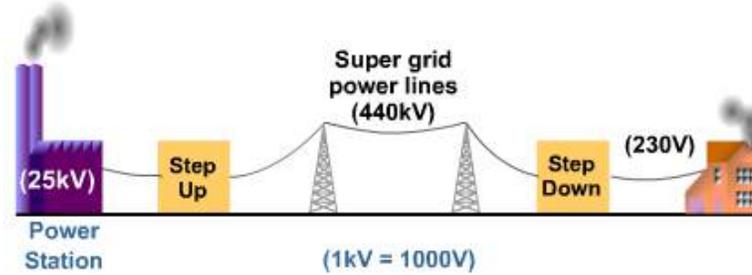
Household electricity has a potential difference of around **230V** and a frequency of **50 Hz (Hertz)**, so changes direction 50 times in a second.
