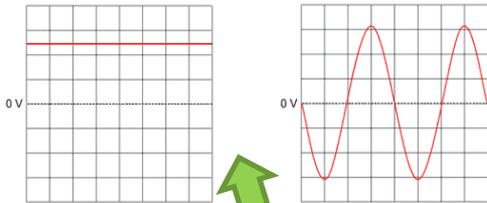
Household electricity has a potential difference of around **230V** and a frequency of **50 Hz (Hertz)**, so changes direction 50 times in a second.
