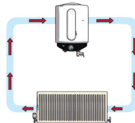
In the boiler and radiator model, the pump pushes the water around the system. It does a similar job to a **battery** pushing the **charges** around a circuit. The pipes carry the flow of water around the system, like the **charge** flowing through wires in a circuit. The radiator is similar to a bulb because it transfers **energy** supplied by the system to the surroundings.
