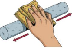
When a polythene strip is rubbed with a cloth, electrons move from the cloth to the strip. The strip becomes negatively charged and the cloth becomes positively charged.
