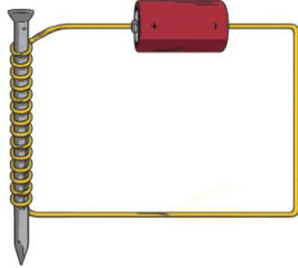
The strength of an electromagnet can be changed by changing the number of coils of wire around the iron core. This can be measured by counting the number of paperclips that become attracted to the electromagnet.
